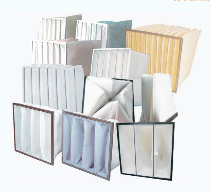
Due to the pocket formation, pocket filters create wide open maximum air entrance into each pocket with minimum resistance. Total pocket inflation results in complete use of media area and offer high dust handling and long service life.
